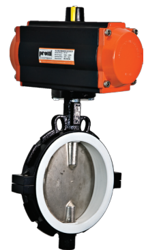
Pneumatic Act. Op. PTFE Seat, AISI316 Disc Butterfly Valve
