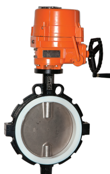
PTFE Seat, AISI316 Disc Electric Act. Op. Butterfly Valve
